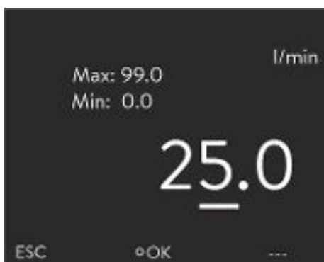
Fig. 51: Setting the flow rate set point
