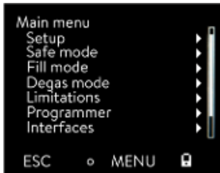
Fig. 71: Operation on the device is locked
