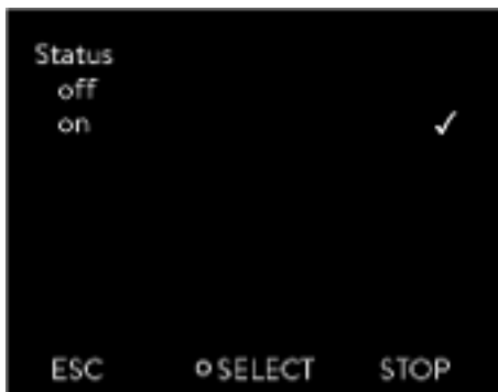
Fig. 48: Flow controller off/on
